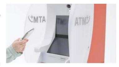
Taking into account the advances in biometrics, AI, IoT, and other technologies, this next-generation ATM is capable of face recognition for identity verification and settlement with QR codes. The machines utilize NeoFace, which is a core technology of Bio-Idiom, NEC's original biometric authentication technologies, to
